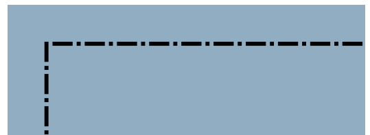
➤ Figure 4: This is a close-up of the dot/dash that results from using a mask value of $A0. See the text for more details of how to come up with other dot/dash patterns.
